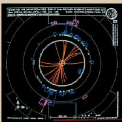
OPAL spots the decay of a Z boson into two jets originating from a quark-antiquark pair
